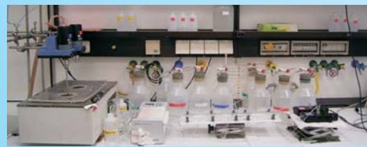
Fig. 2: An autoanalyser system wet alkaline extraction line, for opal content measurement. Water bath, sample vessels and stirrer on the left. A flow through photometer on the right.
