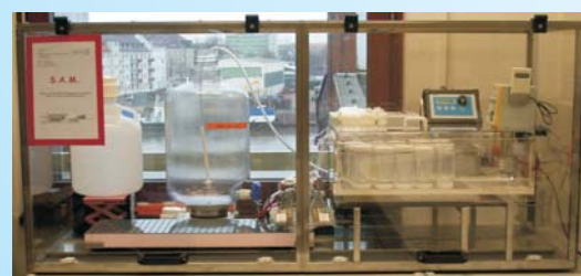
Fig. 4: Photo & schematic illustration of stirred continuous flow-through (CFT) reactor technique coupled with a time-controlled microvalve fraction collector. Inflow solution is added to the reactors with a peristaltic pump. Tygon tubing is used for interconnecting all parts of the system.
