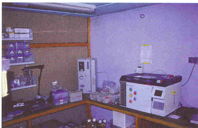
Fig. 6: Laboratory for trace gas analyses (e.g. equipped with a gas chromatograph and a hydrogen generator) and sample preparation for microbiological and pedological analyses (D. Wagner, AWI).
