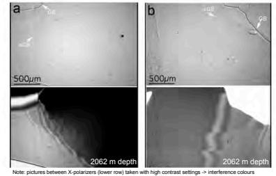
Note: pictures between X-polarizers (lower row) taken with high contrast settings -> interference colours between grains are black and white, whereas sGB show interference differences in grey. Pictures from second EPICA core at Dome C.
