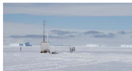
PALAOA , the Perennial Acoustic Observatory in the Antarctic Ocean. A hydrophone array deployed through the 100 m thick Ekström Ice Shelf continuously monitors the underwater soundscape in front of Neumayer Station since January 2006. Recordings contain various marine mammal vocalizations as well as the permanent natural sound background, dominated by the motion of ice.
