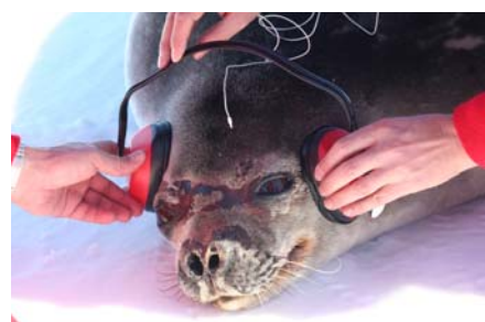
AEP Auditory Evoked Potential measurements were performed on Weddell seals at Atka Bay in December 2005 to obtain basic audiograms. This neuro-physiological technique measures the brain's bioelectric responses to a given acoustic stimulus and allows to determine the audible frequency range and corresponding hearing thresholds of free ranging animals. Furthermore critical sound levels can be estimated from temporary threshold shift (TTS) measurements.
