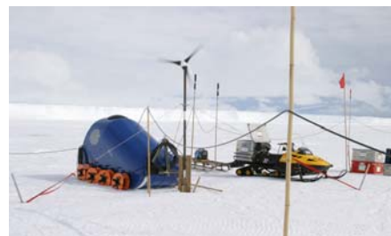
DIPS , Drescher Inlet Pilot Study. A mobile acoustic station in a cabin sledge was set up at the Drescher Inlet, Riiser Larsen Ice Shelf in 2003/04. Three hydrophones, lowered 100 m down through sea ice holes drilled in a 100 m baseline triangle obtained two weeks of underwater recordings, dominated by the local Weddell seal population and Polarstern passings.
