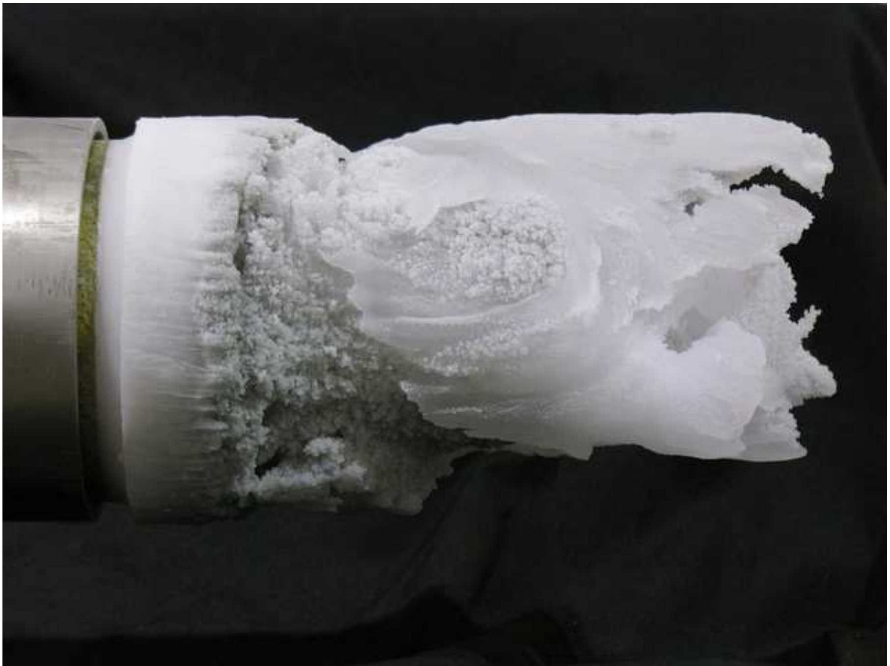
The End of an Ice Core (EDML): refrozen water entering borehole from below
