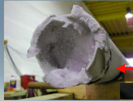
The end of drilling meteoric ice - refrozen water
