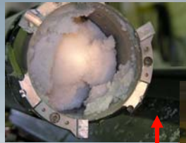
Drilling into the refrozen water: only ca. 30 cm
