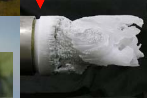
The end of drilling meteoric ice - refrozen water
