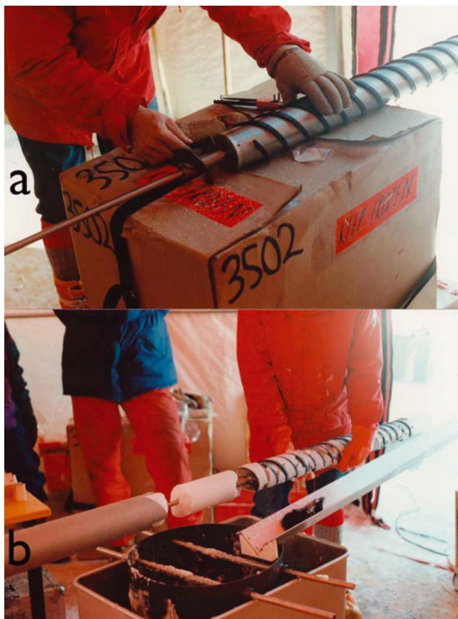
Fig. 1. The modified UCPH shallow drill. (a) Drive shaft, booster and shortened inner core barrel. (b) After a normal successful run, chips chamber, booster and spirals are packed with chips. The chips fall into the black PVC jug with a fine filter at bottom; the liquid is collected in the aluminium bucket.
