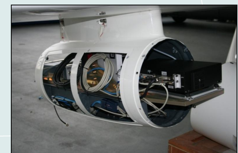
Fig. 2: Sensor and equipment in the wingpod (Photo: OHB).
