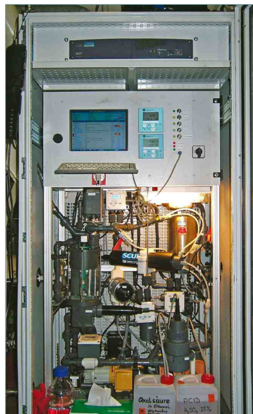
▼ Figure 4 FerryBox System onboard the vessel "TorDania" on the route Cuxhaven - Immingham. Measured parameters: salinity, temperature, turbidity, chlorophyll-a, oxygen, pH, nitrate (UV-detection).
