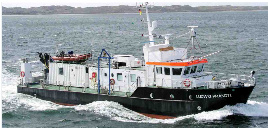
◀ Figure 3 Research vessel “Ludwig Prandtl”, equipped among many other instruments with a downward-looking ADCP for the measurement of water flow and a multibeam echosounder for the observation of the seafloor.
