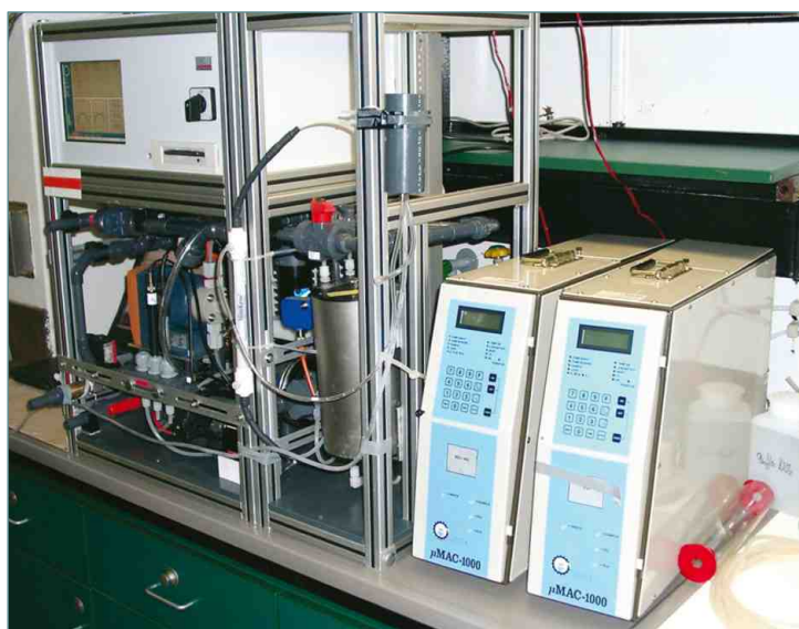
▲ Figure 1 Small version of the FerryBox together with nutrient analysers onboard of the research vessel “Polarstern”.
