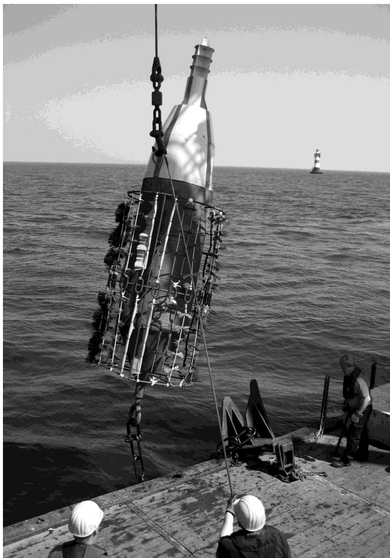
Fig. 3: Modified testing buoyancy equipped with suspended artificial substrates at the offshore sampling site RS at the entrance of the Weser estuary in the German Bight (Brenner et al. 2007).
