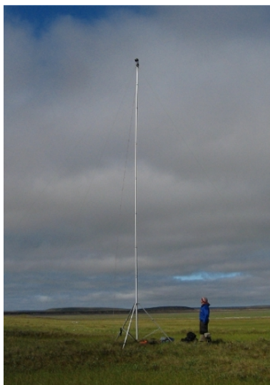
Figure 1.10: The thermal imaging system mounted on the 11 m tower at the field site on Samoylov Island. The thermal imaging system was applied during the summer expedition in 2008.
