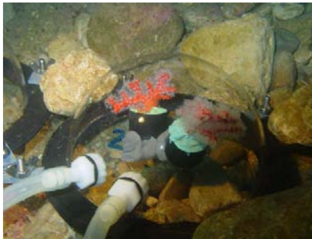
Figure 2: Two red coral colonies in an in situ incubation chamber which is connected to a portable submersible pump (not shown).
