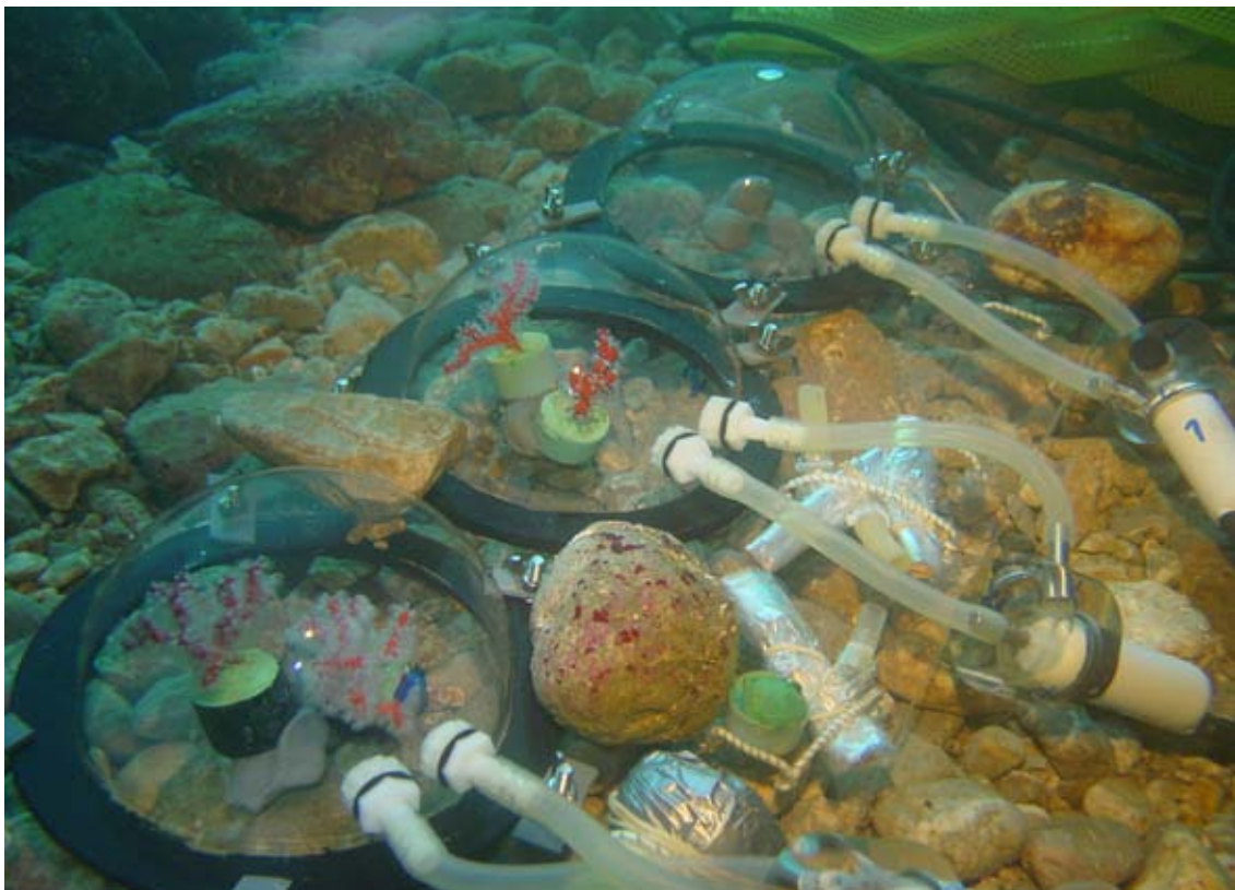
Figure 11: In situ incubation chambers connected to pumps (right hand side) to recirculate the water. The chambers are closed systems allowing to obtain water samples before and after the incubation of the red coral colonies. Note the third chamber is used as control.
