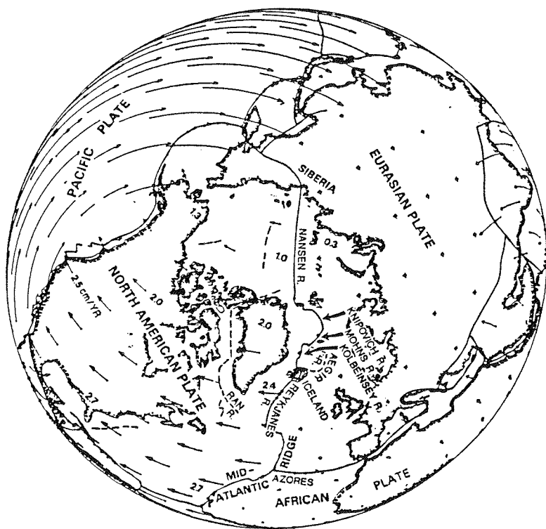
Fig.38 Plate boundary through the Nordic Seas in relation to the adjoining plates and their motions with respect to the deeper mantle. Spreading occurs along some plate boundaries, and slipping or closing occurs along others. The plate boundary between the Azores triple junction and Siberia is the boundary between the Eurasian and North American plates and is the active plate boundary in the Nordic Basin and the Eurasia Basin shown in Fig.2. This figure is redrawn from Minster and Jordan (1980).
