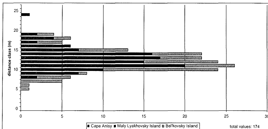
Figure 5.2.13-1: Frequency of distance classes (classes = 1, 2, 3, 4 ... 24, 25 m) for central tops of thermokarst mounds: the values originate from three denudated Ice Complex localities on New Siberian Islands; Most distances from top to top are between 10-15 m, the mean is situated at 12.2 m
