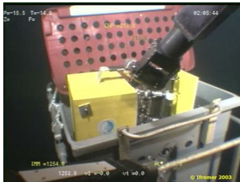
Fig. C2-1: The in situ O 2 micro profiler (MIC) being taken out of the shuttle lander by the ROV.
