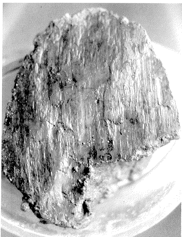
Fig. 1 - Polished and striated slickensided brittle fault surface. Core is 61 mm in diameter.
