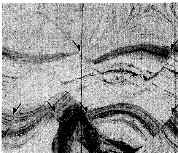
Fig. 2 - Set of 3 normal-sense displacement microfaults in Lower Oligocene strata. Unrolled image of surface of 45-mm diameter whole core. Note the discrete mm-thick fault zones sharply truncate the pre-lithification folds. Arrows denote apparent sense of motion. Discrepancies in magnitude of apparent offset of layers across the fault are attributed to displacement of layers with variable dips and thicknesses due to the soft-sediment folding.
