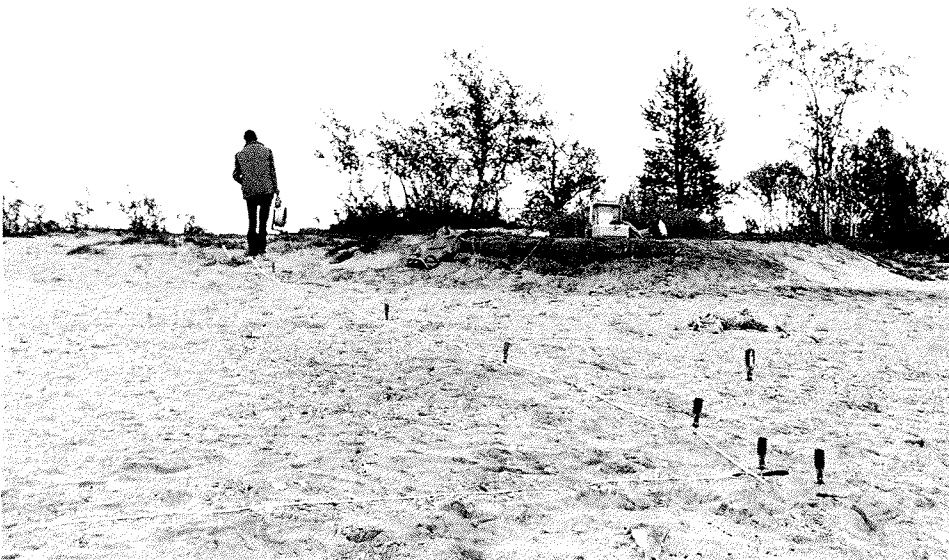
Fig. 14: Sounding site at a large deflation surface on the edge of Peldojoki glaciofluvial delta. Steel probes M/N are in the foreground, the electrode sticks may be recognized along the measuring tape. The recording instruments are located on a small terrace. Photographed by M. Seppälä, August 5, 1985.
