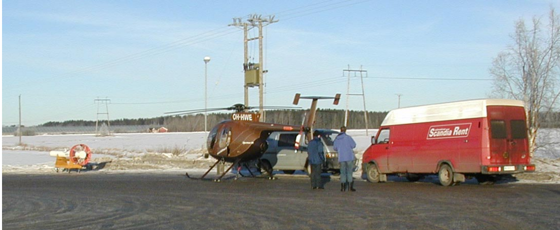
Figure 6: Photograph of the ground logistics, consisting of (from left to right): EM bird on trolley, MD-500 helicopter, refueling truck, and scientist equipment van.
