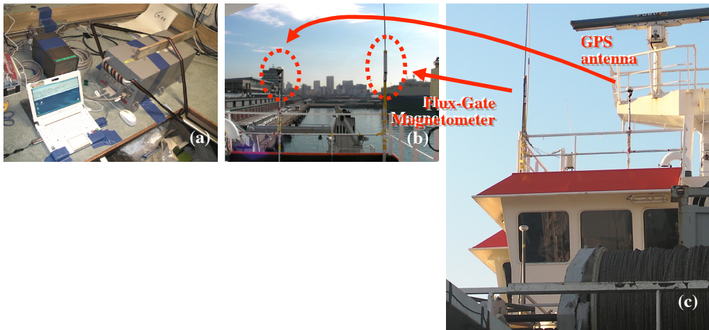
Fig. 18: Pictures of the STCM system on RV Pelagia. (a) RLG, controller and laptop computer in the CTD room; (b) + (c) FG sensor and GPS antenna are attached on the top deck above the bridge.
