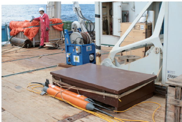
Fig. 10 above: GPS-antenna used for gradiometer system. Below: gradiometer sensor
