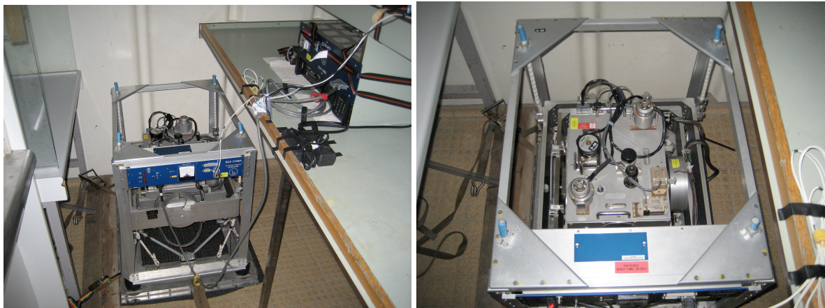
Fig 13 a + b: S56 Sea gravimeter installed on RV Pelagia
