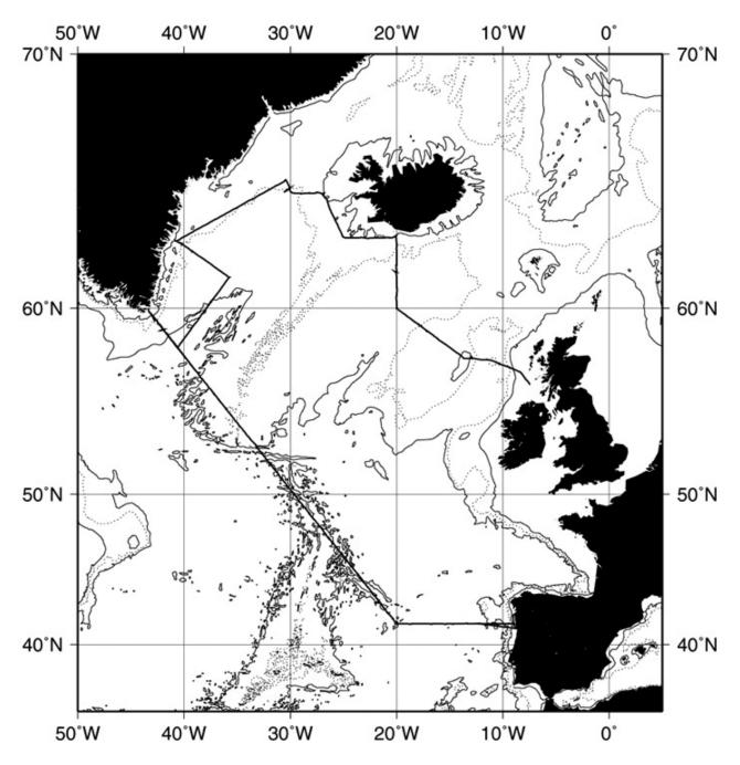
Figure 1.1: *Discovery* Cruise 230 track Vigo to Southampton. Bathymetry is 200m (solid), 1500m (dots), 3000m (solid).
