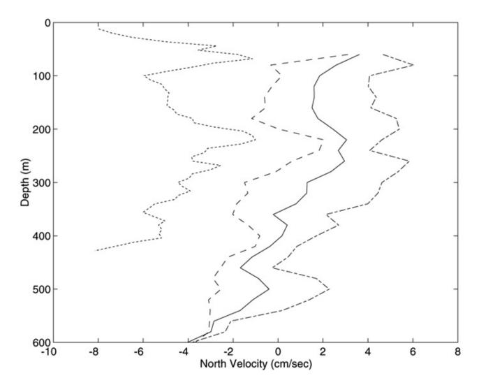
Figure 3.1: VM- and L-ADCP profile comparisons for station 85; VM-ADCP: short dash; L-ADCP: down (chain), up (long dash), mean (solid).
