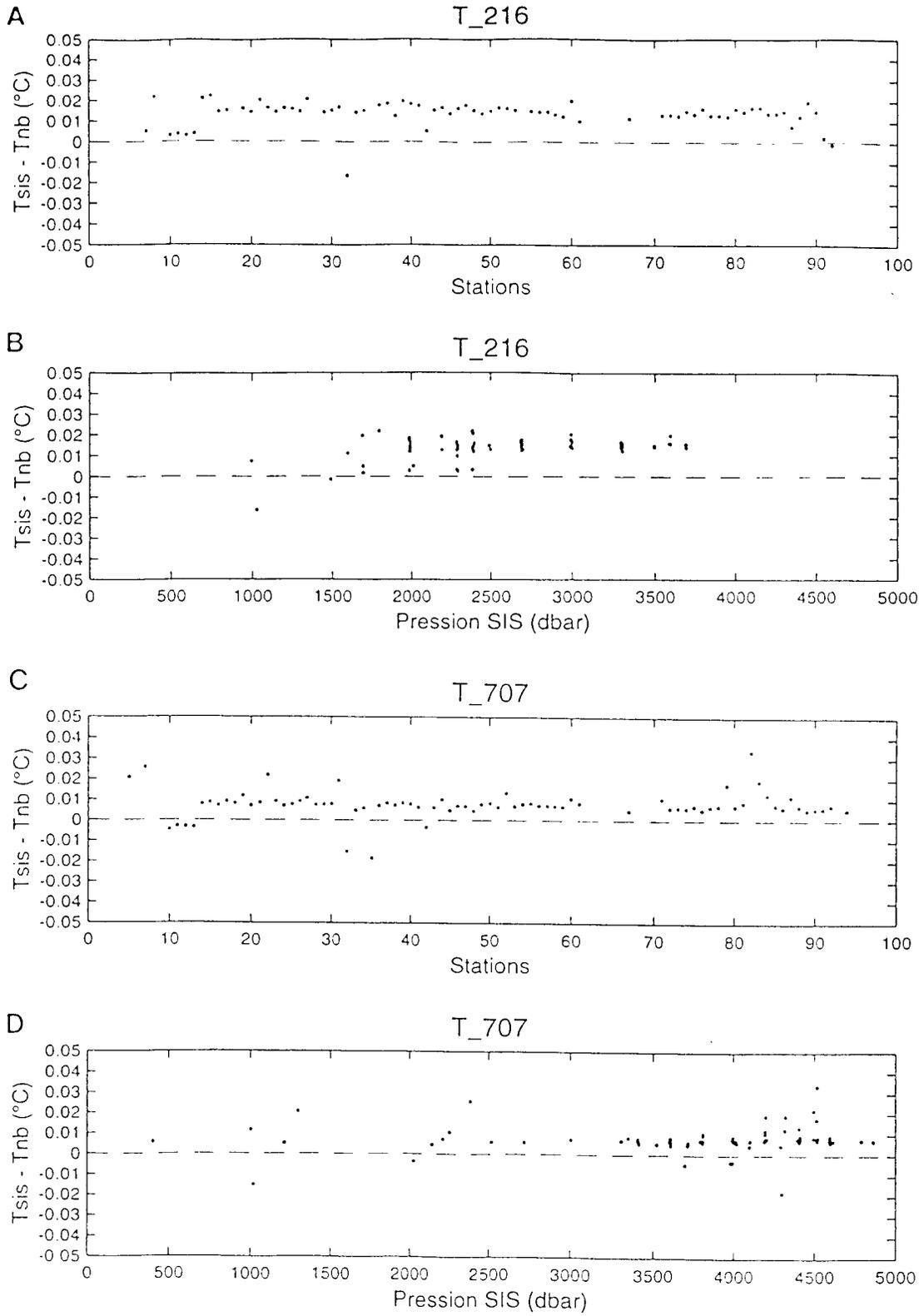
Figure 6: Temperature difference, in  $^{\circ}C$ , between SIS and CTD measurements (after calibration).
