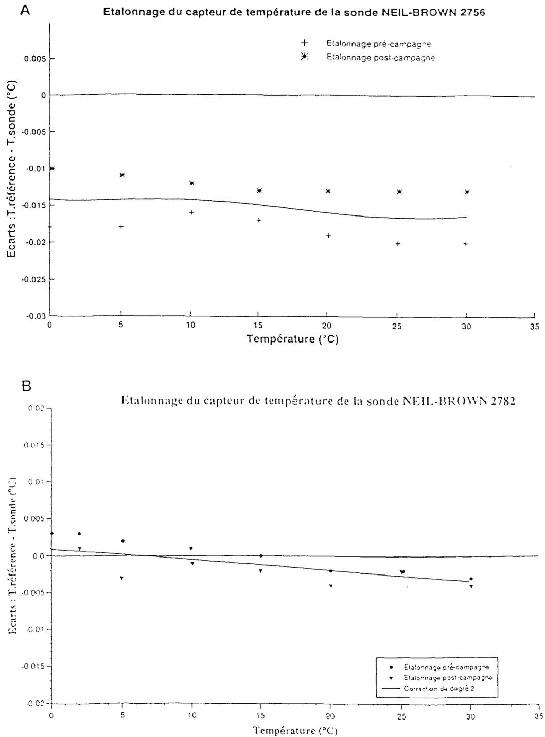
Figure 5: Temperature difference , in °C, between the laboratory reference temperature and the temperature measured by the probe. The solid represent the 5<sup>th</sup> order polynomial minimizing the differences.
