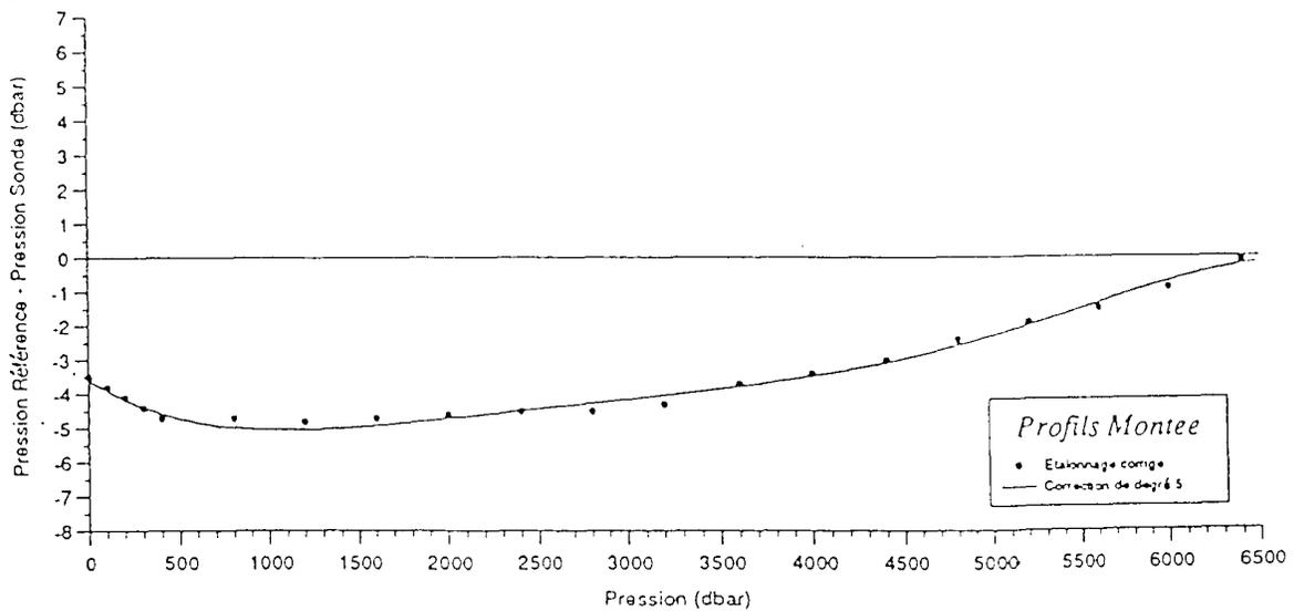
Figure 8: Calibration curve for the pressure sensor of the N°2782 CTD probe
