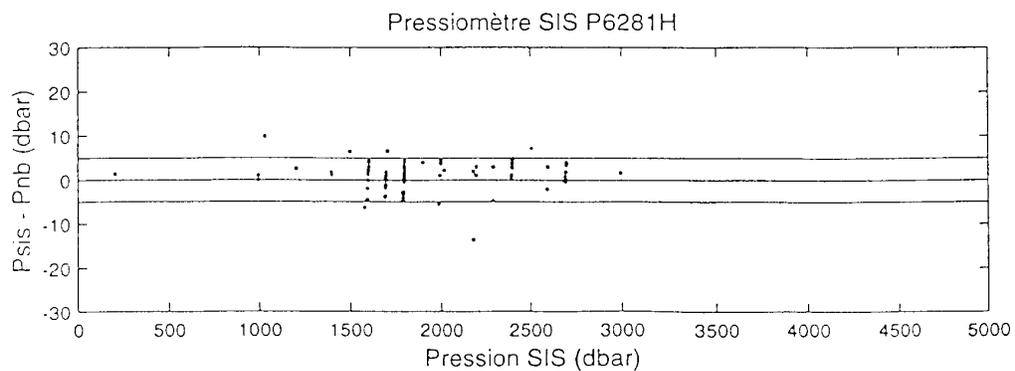
Figure 9: Pressure difference, in dbar, between SIS and CTD measurements (after calibration).
