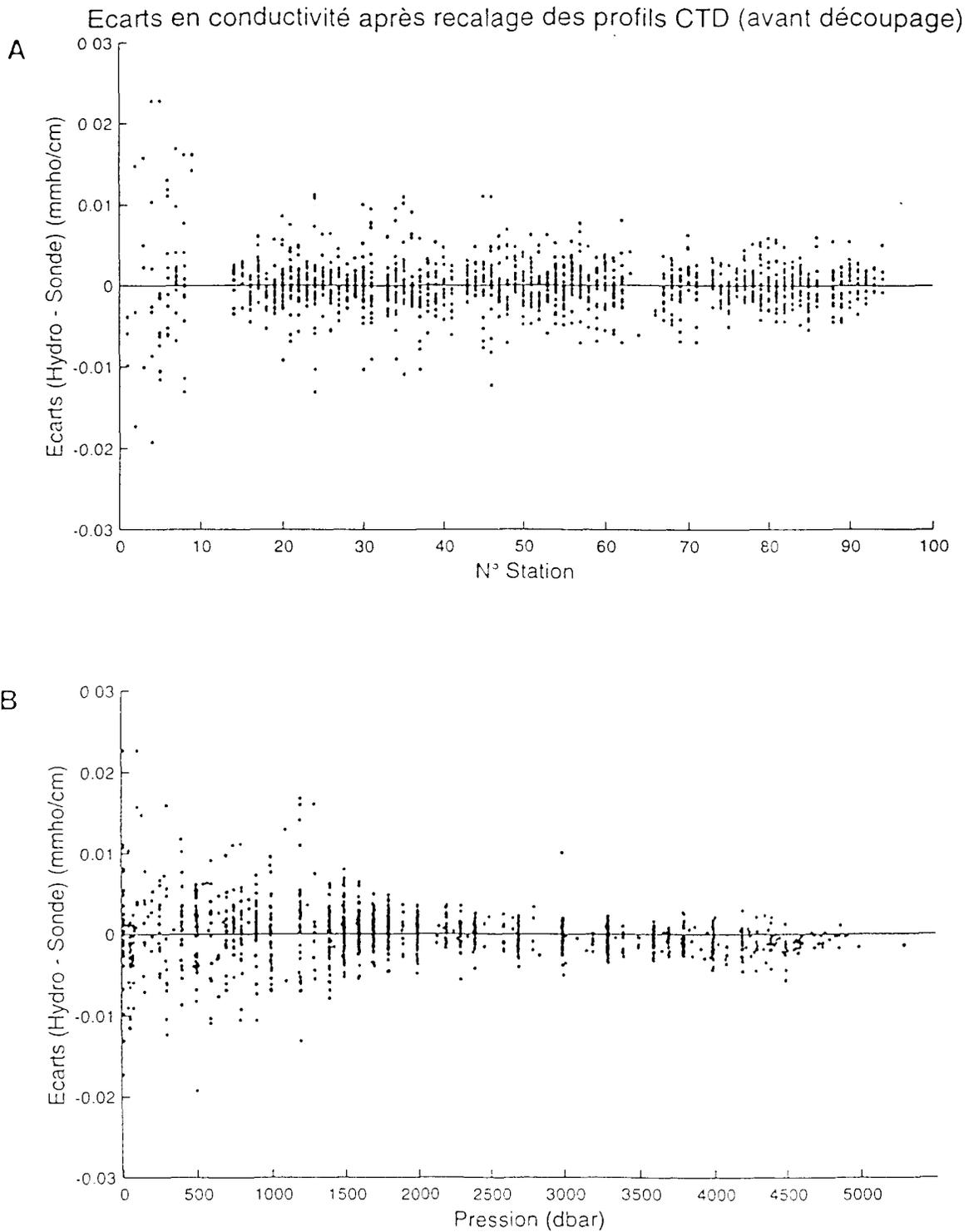
Figure 10: Conductivity difference, in mmho/cm, between water sample and CTD measurements, after calibration.
