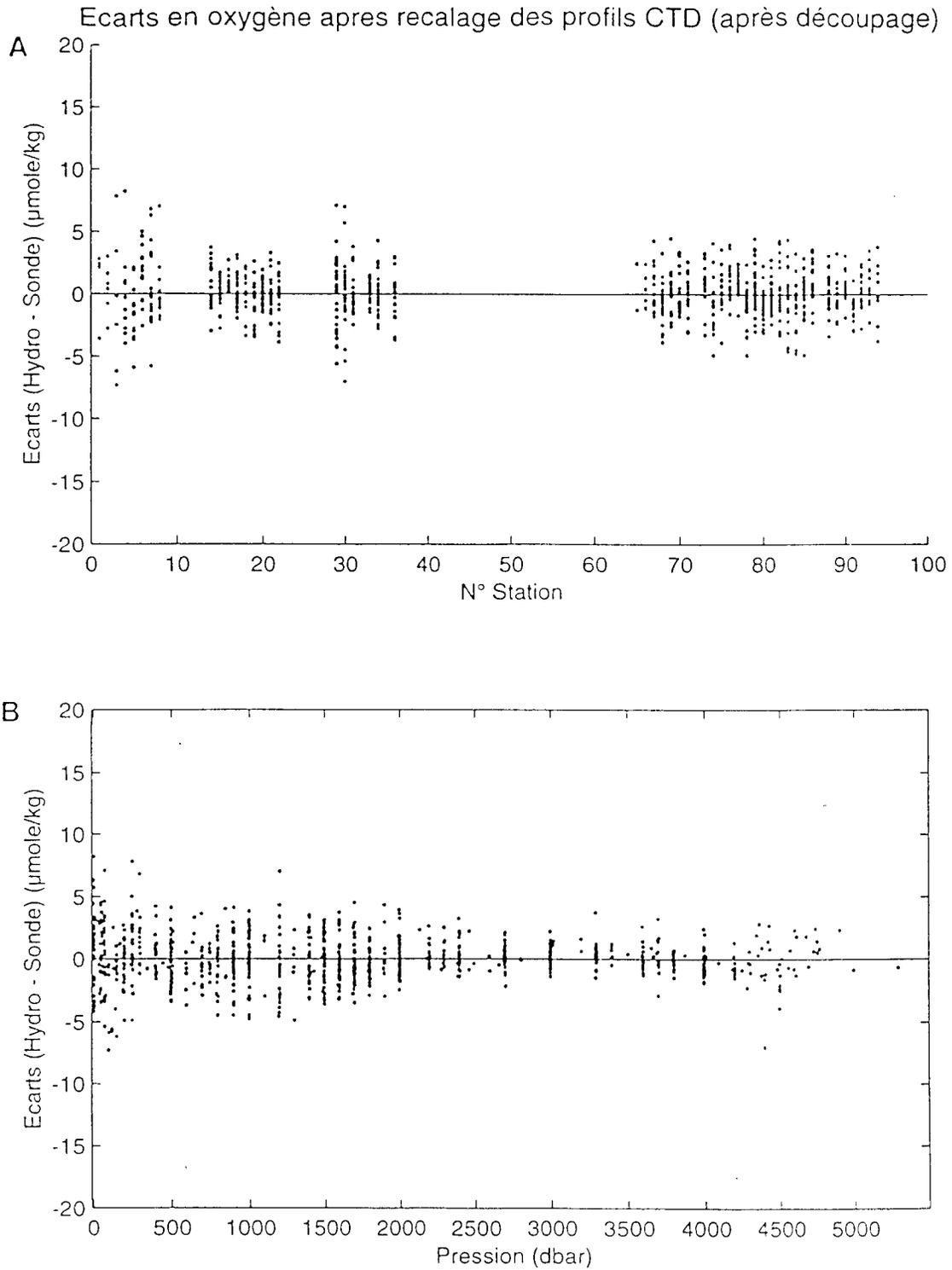
Figure 12: Dissolved oxygen difference, in  $\mu \text{ mol kg}^{-1}$ , between water sample and CTD measurements.
