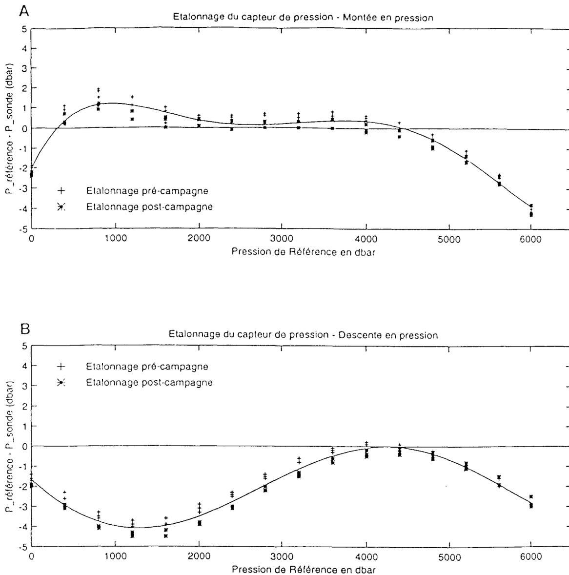
Figure 7: Pressure difference, in dbar, between the laboratory reference pressure and the pressure measured by the N°2756 probe. The solid represent the 5<sup>th</sup> order polynomial minimizing the differences.
