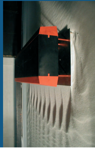
A model of the Neumayer Station III in the wind tunnel of the Meteorological Institute, University of Hamburg
