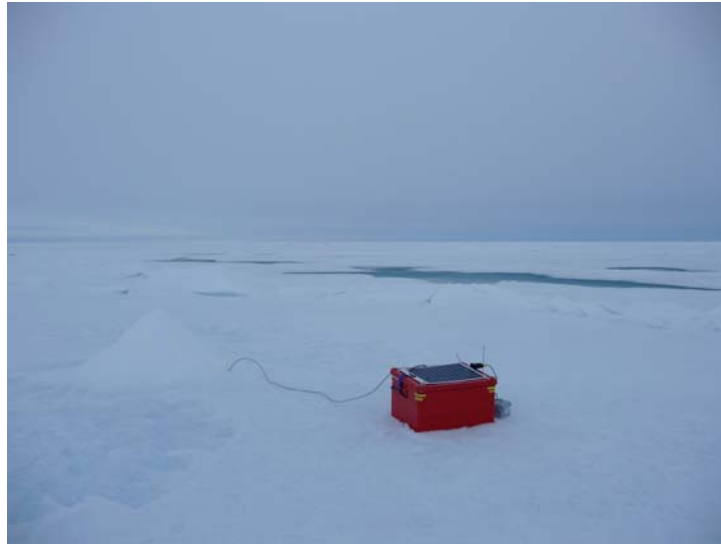
Fig. 3.2.2: Picture of station Lena1-2 after deployment. The seismometer is covered by a plastic bucket and snow to protect it from temperature changes. The Reftek datalogger and the batteries are stored in the red Zarges box. Argos transmitter and the antennas of GPS and Argos are visible at the right side of the Zarges box. Note the solar panel mounted on the Zarges box.
