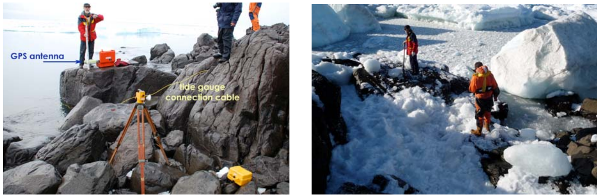
Fig. 4.2: Set up of the SHAN tide gauge station. Left: The instantaneous sea level height is determined with respect to a GPS antenna. The tide gauge itself consists of a small pressure sensor that is directly put into the water, and which is connected with a small data recorder stored at the coast. Right: Shannon tide gauge site at time of the re-collection of the equipment
