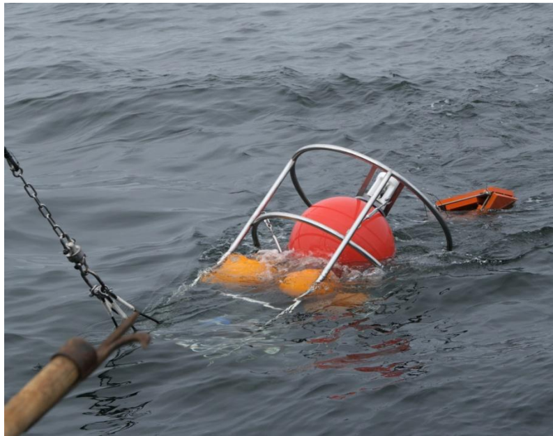
Figure 4: Recovery of the winch and profiling body after the first deployment.
