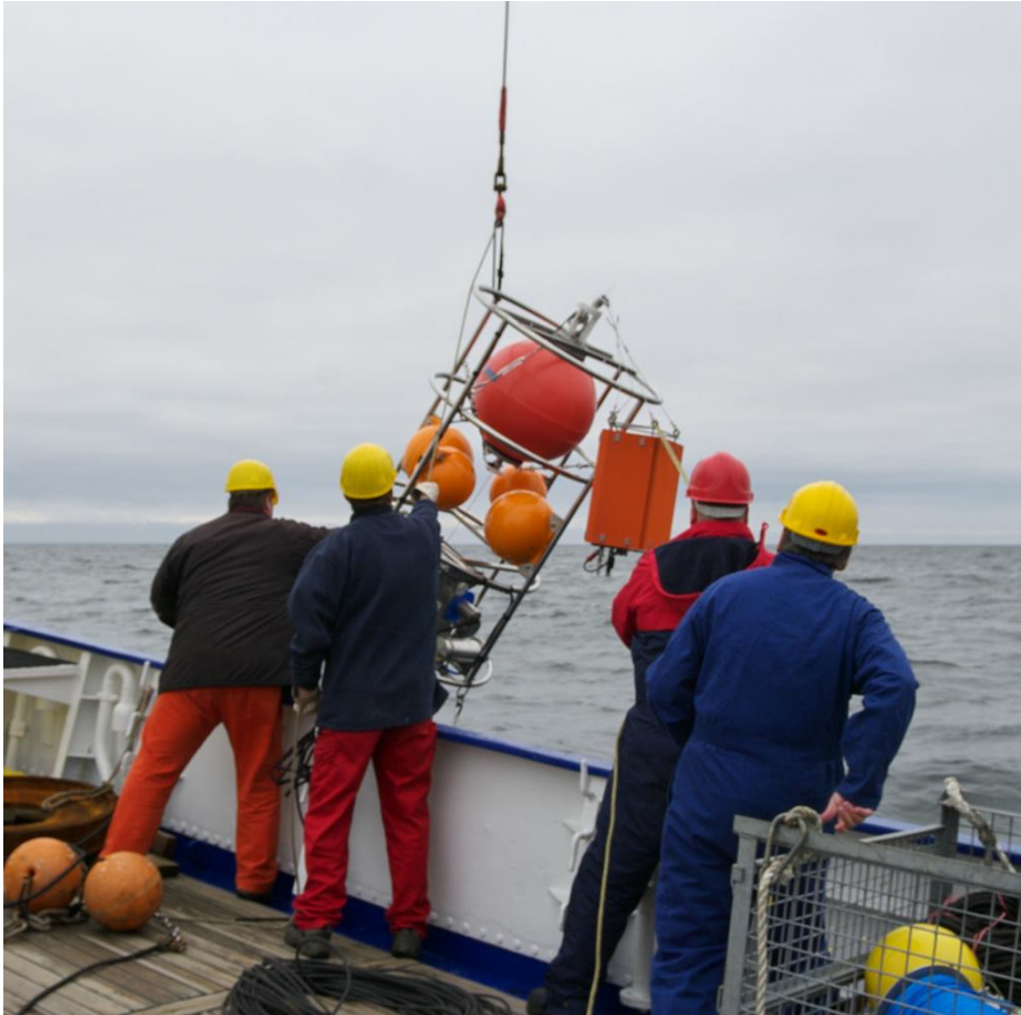
Figure 3: Deployment of the winch and profiling body for the first trial. The profiling body is upside down as it only rights itself due to the buoyancy in the water. (Photo D. Meyer)
