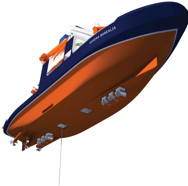
Fig. 4: Special hull shape with forward propulsion and transverse thrust units. Note the placement of the twin moon pools between the transverse thruster units. The swath bathymetry and sediment echo-sounding systems are placed before the forward transverse thrusters in the protruding ice keel.
