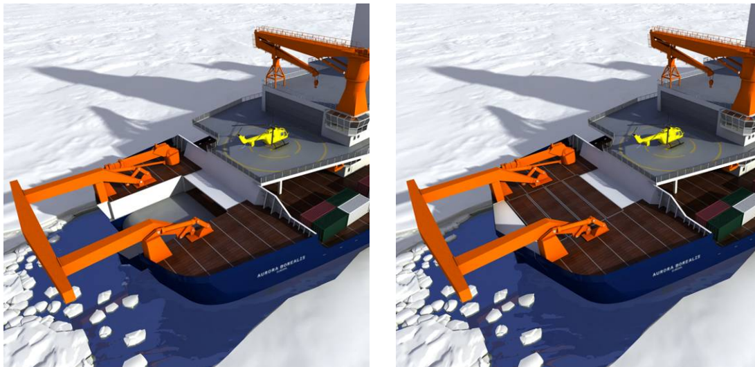
Fig. 13: rear view with stern chutes, A-frame, helicopter pad and hangar, left side: cover piece removed and stern chute opened, right side: fully closed stern section.
