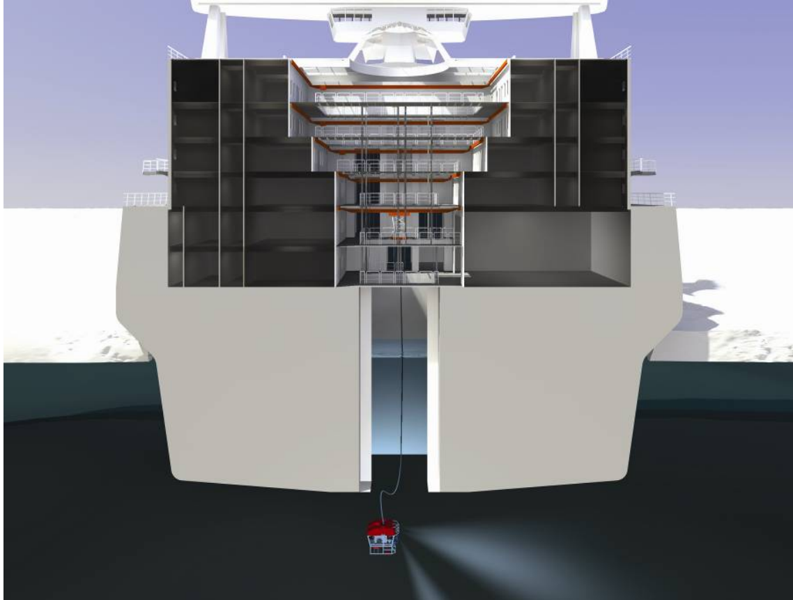
Fig. 8: Cross section through AURORA BOREALIS – Fore moon pool with atrium and cupola roof as well as lateral icebreaking flanks
