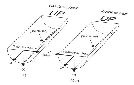
*Figure 1—1 Core orientation conventions.*
