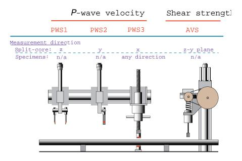
Figure 1—2 Schematic view of the semiautomated instrumentation on the working-half core track. n/a = not applicable.
