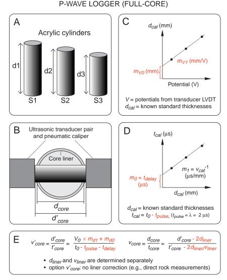
*Figure* 6—2 *Schematic of PWL calibration. A. Physical standard used. B. Measurement geometery. C. and D. Calibration principle. E. Application of calibration to core measurement.*
