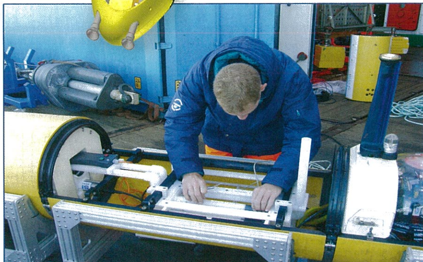
(Below) During preparation for the next dive, the sample tubes are inserted.
