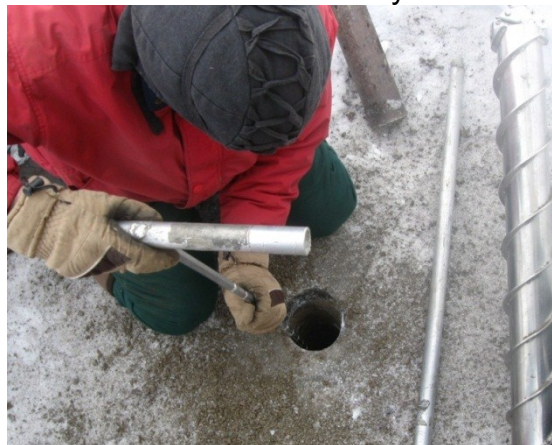
Fig. 1.22: Drilling with an SIPRE-Corer at the top of the Yedoma hill. Picture by K. Bjella (May 2012)
