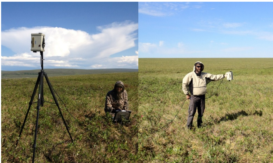
Fig. 3.15: Set-up for the spectro-radiometric measurements (here: device check). Left: irradiance measurement; Right: radiance measurement of the target (simultaneously with the irradiance measurement). Pictures by M. Buchhorn and M. Schwieder.
