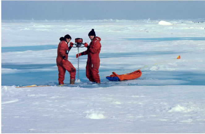
Fig. 7: Top: Drilling in a melt pond for ice thickness measurements (Photo: W. Dierking). Bottom: ice thickness measured during the cruise ARK-VIII/3 (ARCTIC 91) The ice thickness was either measured along 50 m long profiles or on different ice floes accessed by helicopter (from FÜTTERER 1992).
