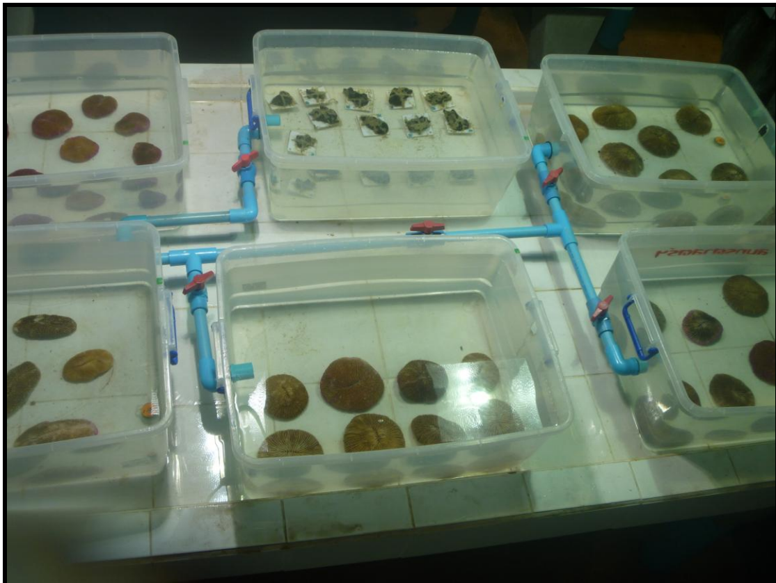
Fig. 5: The flow- through system with corals and sponges.
