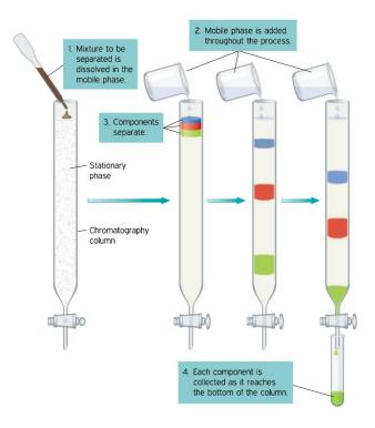
**Figure 1.9:** Schematic of silica or alumina column chromatography to separate a mixture of organic compounds into different fractions prior to analysis. (Figure from explow.com/chromatography)
