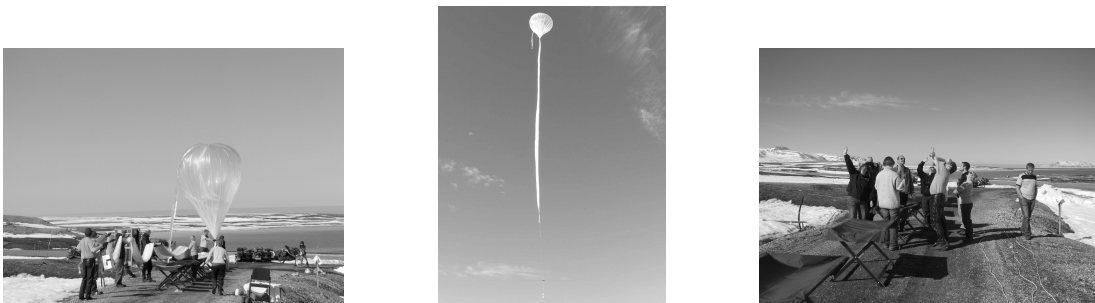
Figure 6.4: Launch preparation of a polyethylene balloon: unfurling of the balloon-rest and start of the sonde.
