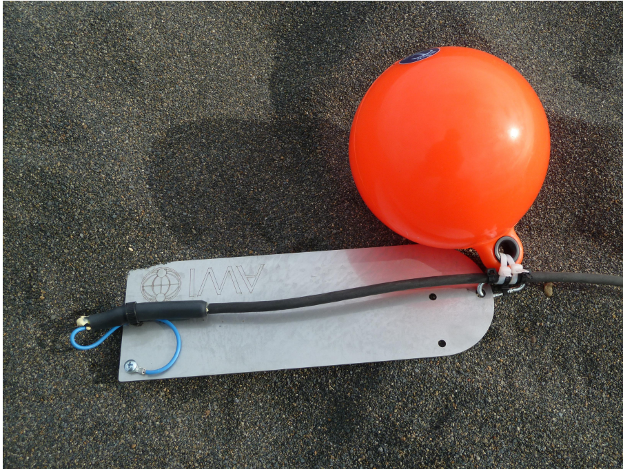
Fig. 6.1: An example of an electrode, in this case at the end of the electrode cable, take-out and buoy.
