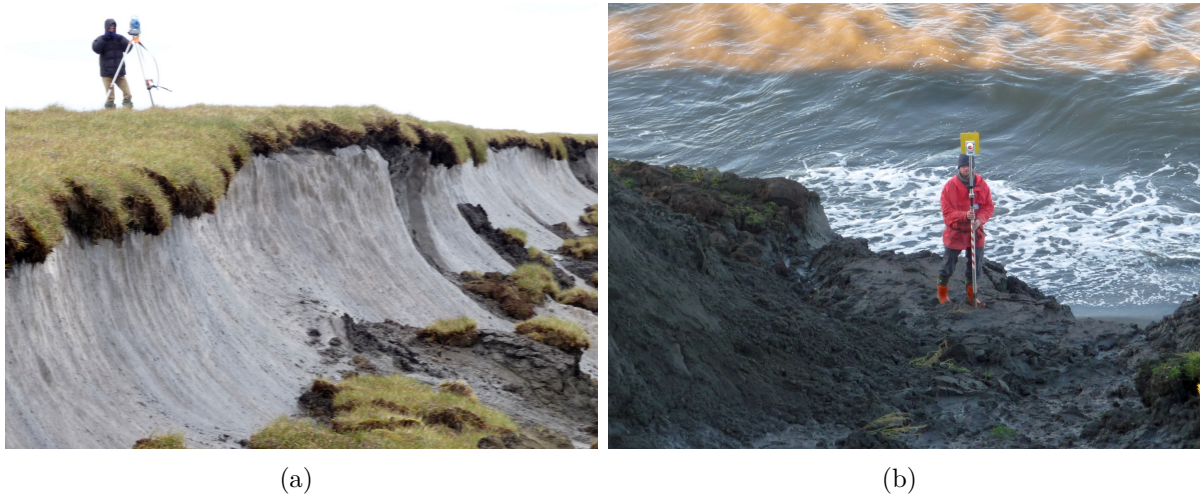
Fig. 4.1: Methodological setup of topographic surveys: (a) tacheometer operator on coastal cliff top near navigation sign Mamontov Klyk; (b) reflector mirror operator on a coastal slope.
