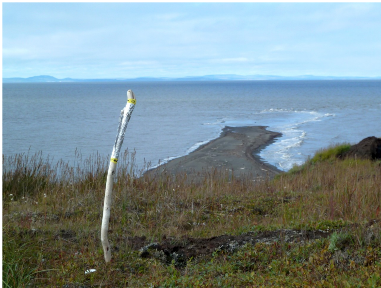
Fig. 4.2: Fixed and marked backside point (№ 29) near the northern cape and adjacent sand spit of Muostakh. Backside points can be used for repeat surveys during following expeditions in order to support consistent instrument positioning.
