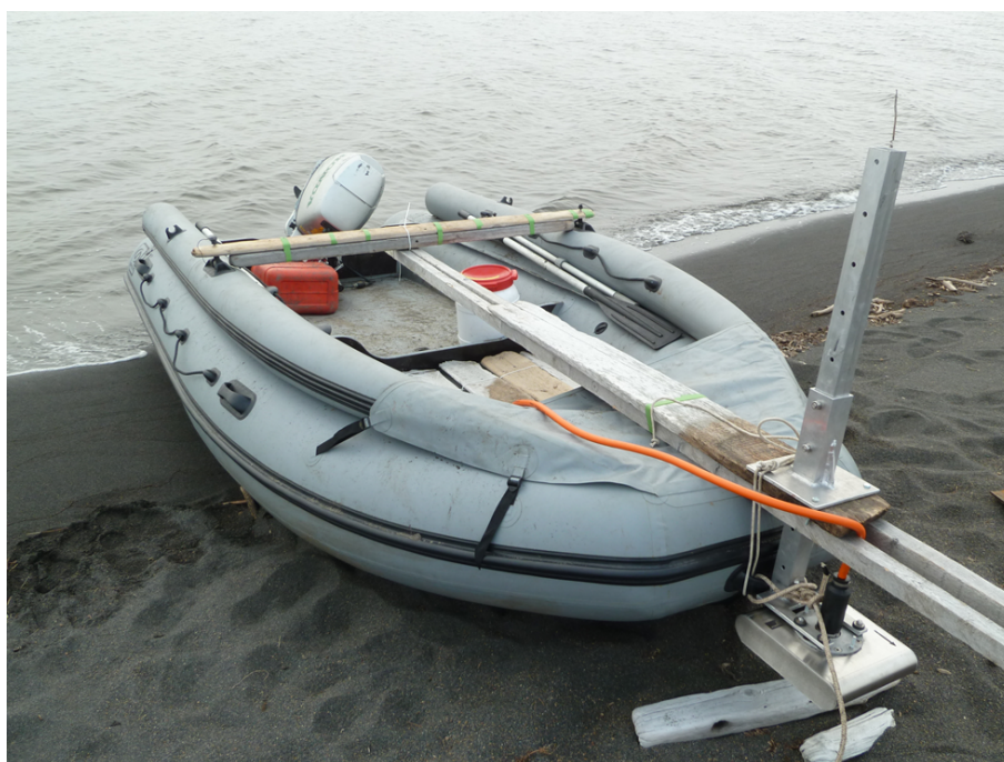
Fig. 6.4: The inflatable dinghy is shown with improvised sub-bottom profiler transducer mount at the bow.
