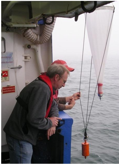
Plankton net, pore size 20 \mu\text{m}
