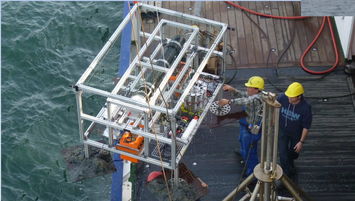
Deployment of the under water gas analyser system
