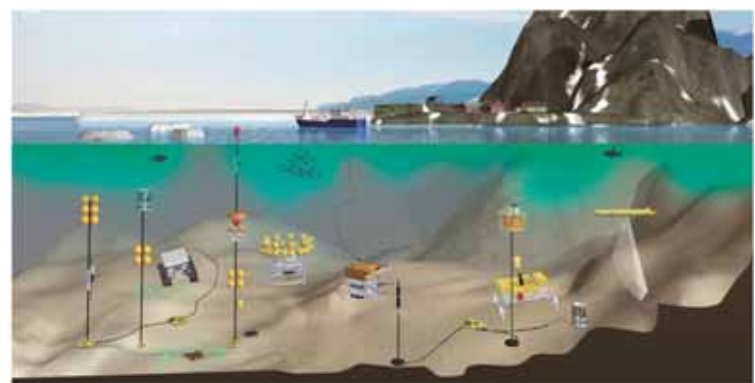
Artist's vision of FRAM: a multi-component, multi-disciplinary observatory for year-round observations of physical, chemical, and biological ecosystem components (Sabine Lüdeling, www.medieningenieure.de).
