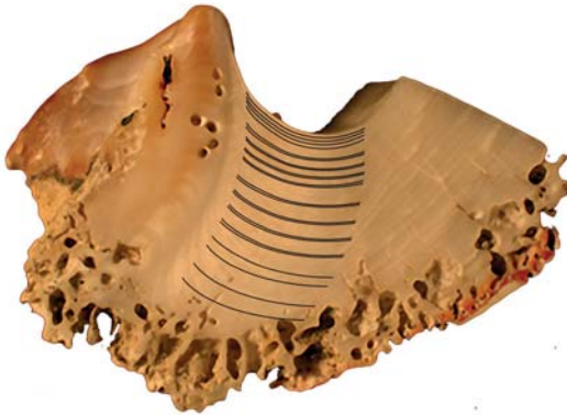
Fig. 7: Simplified scheme of our automated milling lines, starting with lines very close to each other at the most recent formed parts of the shell and then moving further outside to the oldest parts of the shell with wider growth bands where we also increased the distance between the milling lines. We sampled twice per growth band: one sample from the opaque and one sample from the translucent part.
