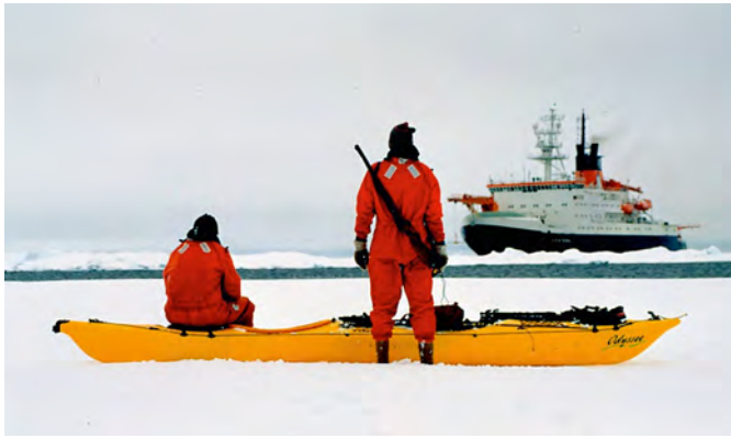
Fig. 11: Ice thickness measurements during ARK XVII/1, using a ground-based EM instrument housed in a kayak (Photo: J. Bareiss).
