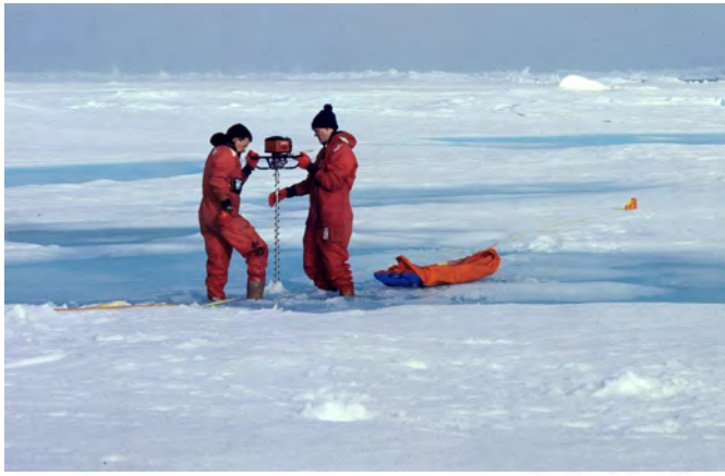
Fig. 7: Top: Drilling in a melt pond for ice thickness measurements (Photo: W. Dierking). Bottom: ice thickness measured during the cruise ARK-VIII/3 (ARCTIC 91) The ice thickness was either measured along 50 m long profiles or on different ice floes accessed by helicopter (from FÜTTERER 1992).
