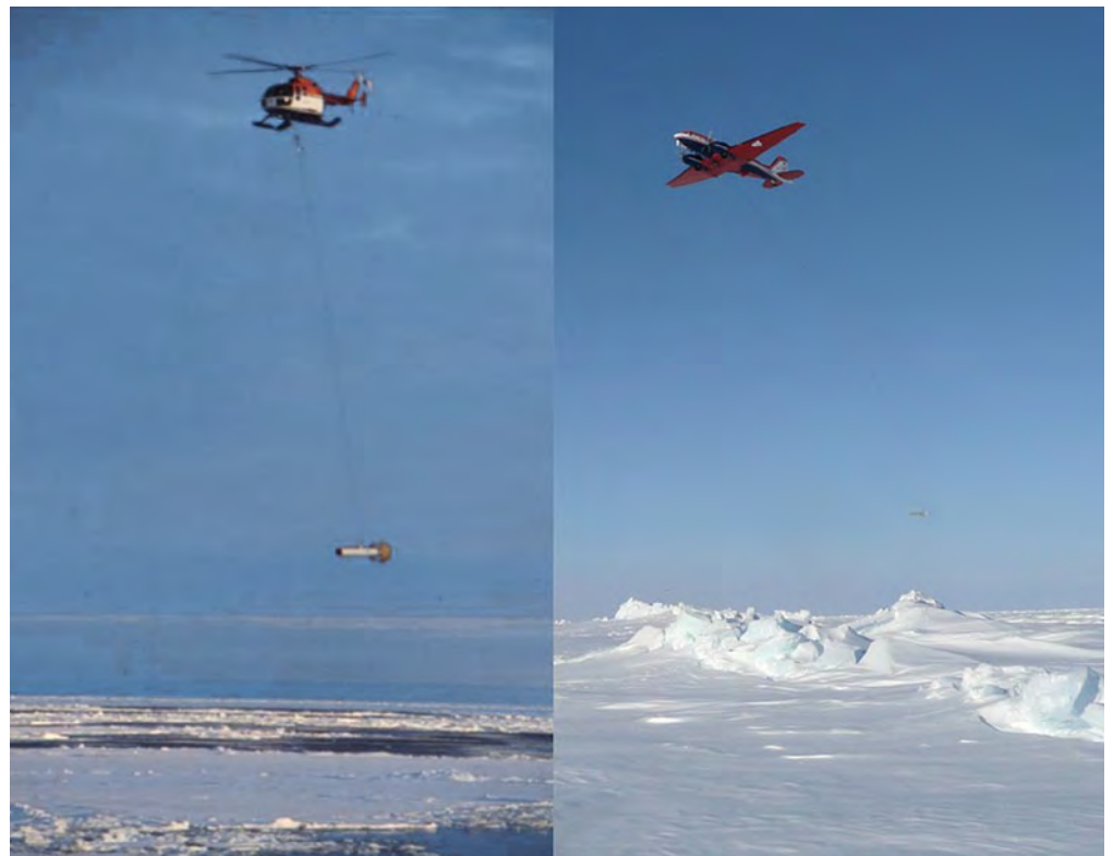
Fig. 12: Left: First flights with the EM-bird in the central Arctic Ocean in 2001. The bird is flown by helicopter 15 m above the ice surface (Photo: J. Lieser). Right: Since 2009, airborne EM ice thickness surveys are conducted with AWI’s “Polar 5” airplane (Foto: C. Haas).
