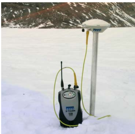
Figure 3.10 The position of ablation stakes in 2010 was measured by DGPS. The GPS receiver is shown configured with a VHF antenna for RTK-GPS, but post-processing had to be used because VHF signal coverage was poor. Photo: Michele Citterio, GEUS.
