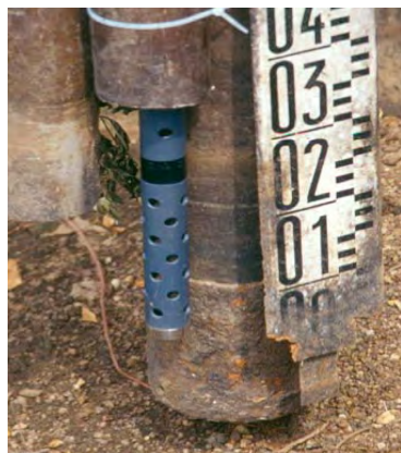
Fig. 5.5 Turbidity probe after installation in the river bed
