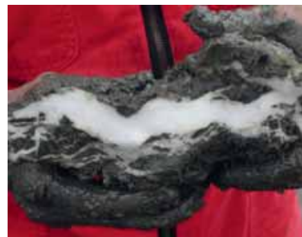
White gas hydrates consolidate sea floor sediments
