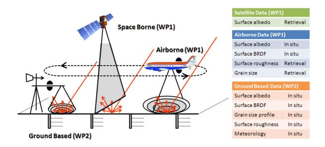
**Figure 1:** Illustration of measurement strategy including ground based (work package WP2), airborne (WP1) and space borne (WP1) measurements of optical and microphysical surface characteristics. (Illustration by A. Ehrlich)
