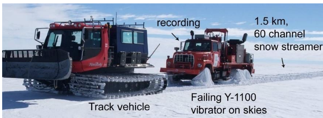
Fig. 25; the PistenBully pulled the vibroseis source, which was mounted on skis, after that the snowstreamer. From Kristoffersen et al. (submitted).
