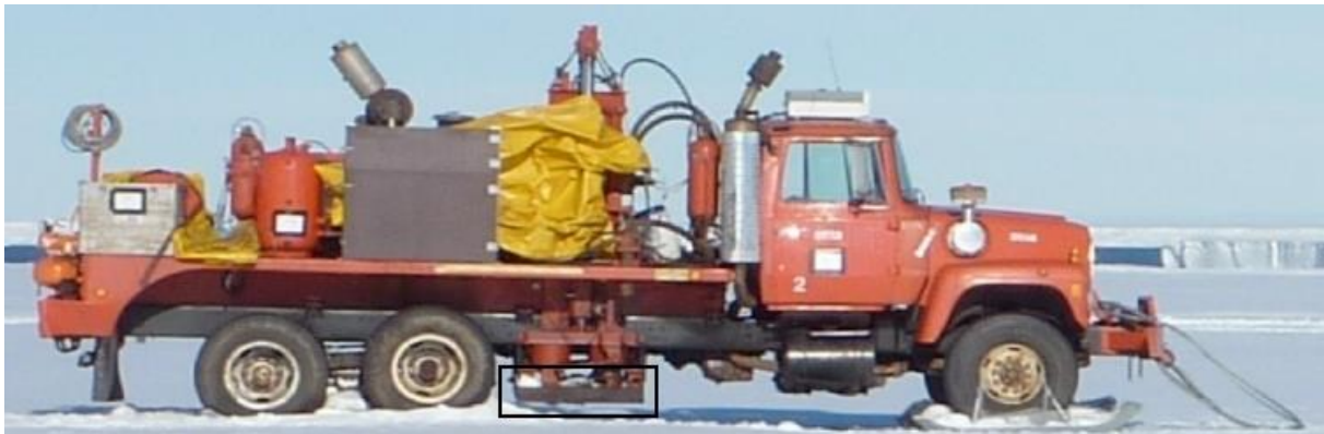
Fig. 12; a truck-mounted vibrator, the black rectangle marks the plate, which will be lowered down. Photo from Lambrecht et al. (2010).
