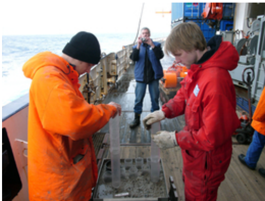
Sampling the seafloor with a box corer.
