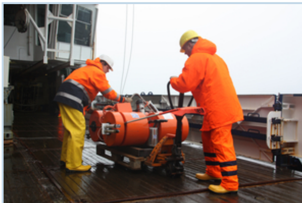
OBS on its way Crew and scientists move the ocean bottom seismometer to the working deck. Photo: Folke Mehrtens, Alfred Wegener Institute
