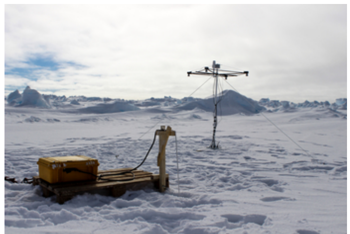
Fig. 2: The Ice Mass Balance Buoy (yellow Pelicase) is used to calculate the sea ice growth; the snow depth buoy (background) measures the changes in the snow height. © S.Schwegmann (AWI)
