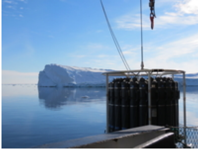
Fig. 3: The CTD rosette is launched in front of a fantastic landscape. The device measures water temperature, salinity and conductivity, and collects water samples from different depths. © Svenja Ryan (CAU)
