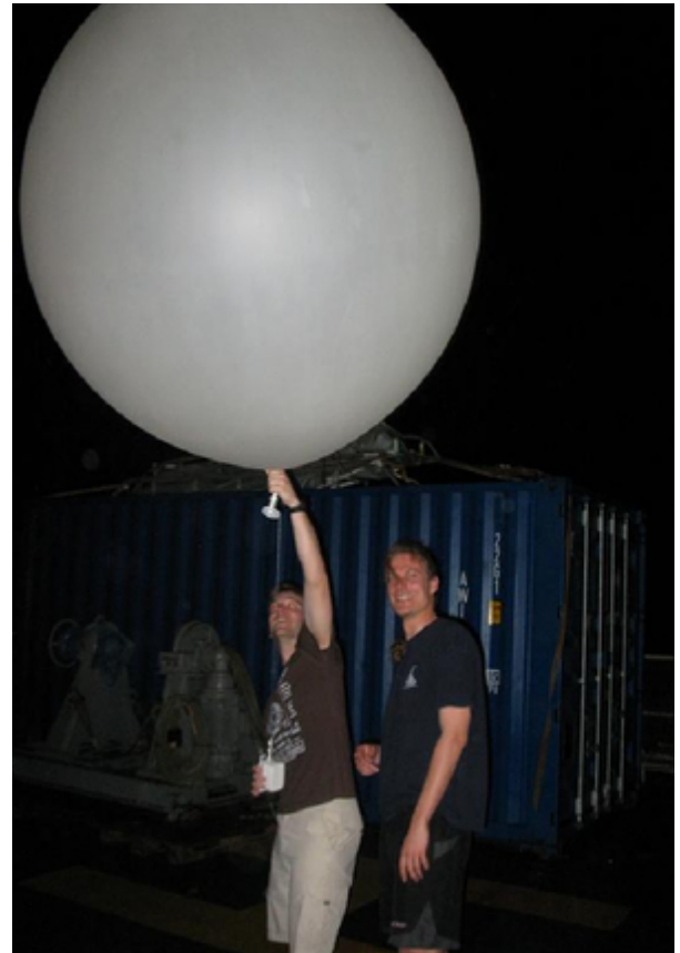
Launch of a radiosonde at night. During the ascend of the probe meteorological data are transmitted to the ship. (© T. Hanschmann, IFM-GEOMAR)
