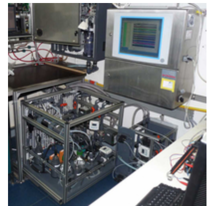
Fig. 4: Newly installed FerryBox (foreground) together with its control unit (up right). (photo: St. Aßmann)
