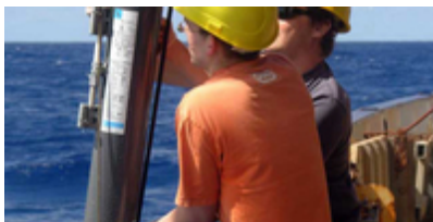
Fig. 2: Thibaut Wagener (left) and Diego Gaiero take water samples with a special GOFLO sampler. (photo: A. Körtzinger)
