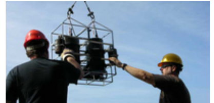
Fig. 4: R. Reynolds (right) deploys an instrument package containing sensors for spectral backscattering and a Laser diffraction instrument for in-situ measurements of particle size distribution.
